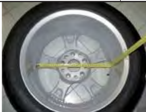
Figure F3.3.1 Example of manual measuring of the external diameter (da2) of the wheel in the ALS1/ALS2 Program Type
