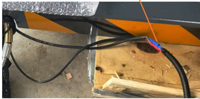
Connect the LOCK button wire from control panel to the mating connection coming out of the scissor lift.
