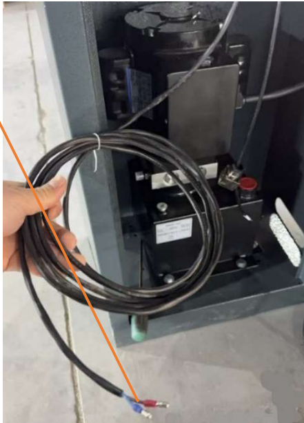
Connect the LOCK button wire from control panel to the mating connection coming out of the scissor lift.
