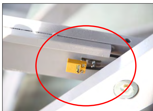
Picture 17 (lower limit switch)
