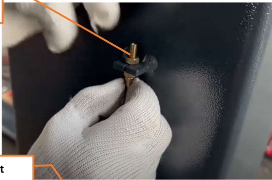
Install the cable tensioner on the power side post
